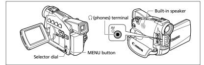
When using the built-in speaker, make sure that " $\Omega$ " is not displayed on the screen. When using the headphones, make sure that " $\Omega$ " is displayed. Change the setting as necessary following the procedure below.
